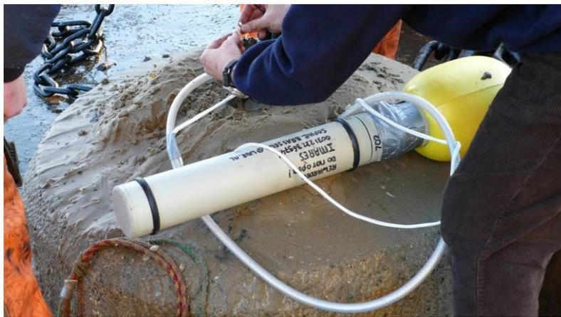
Figure 8: T-POD about to be deployed at position AT\_5 in the OWEZ
