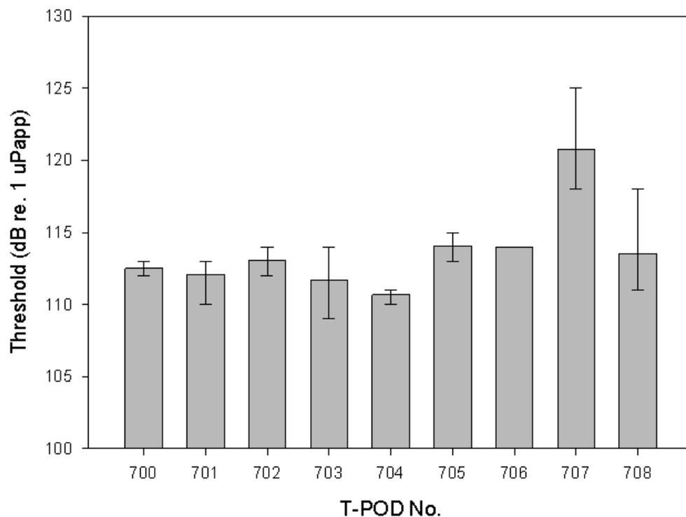
Figure 1: Results of the tank calibration of the T-PODs (v5) used during the  $T_1$  study
