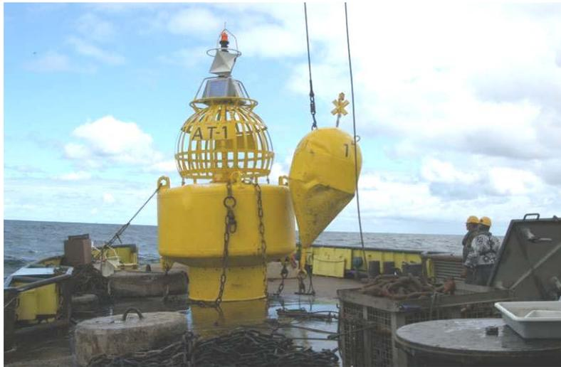
Figure 7: T-POD being attached to the anchoring system. The Kevlar line is reinforced with rubber tubing and a PVC foam float is attached at the top of the T-POD to increase the buoyancy (see appendix 3 for sketch).
