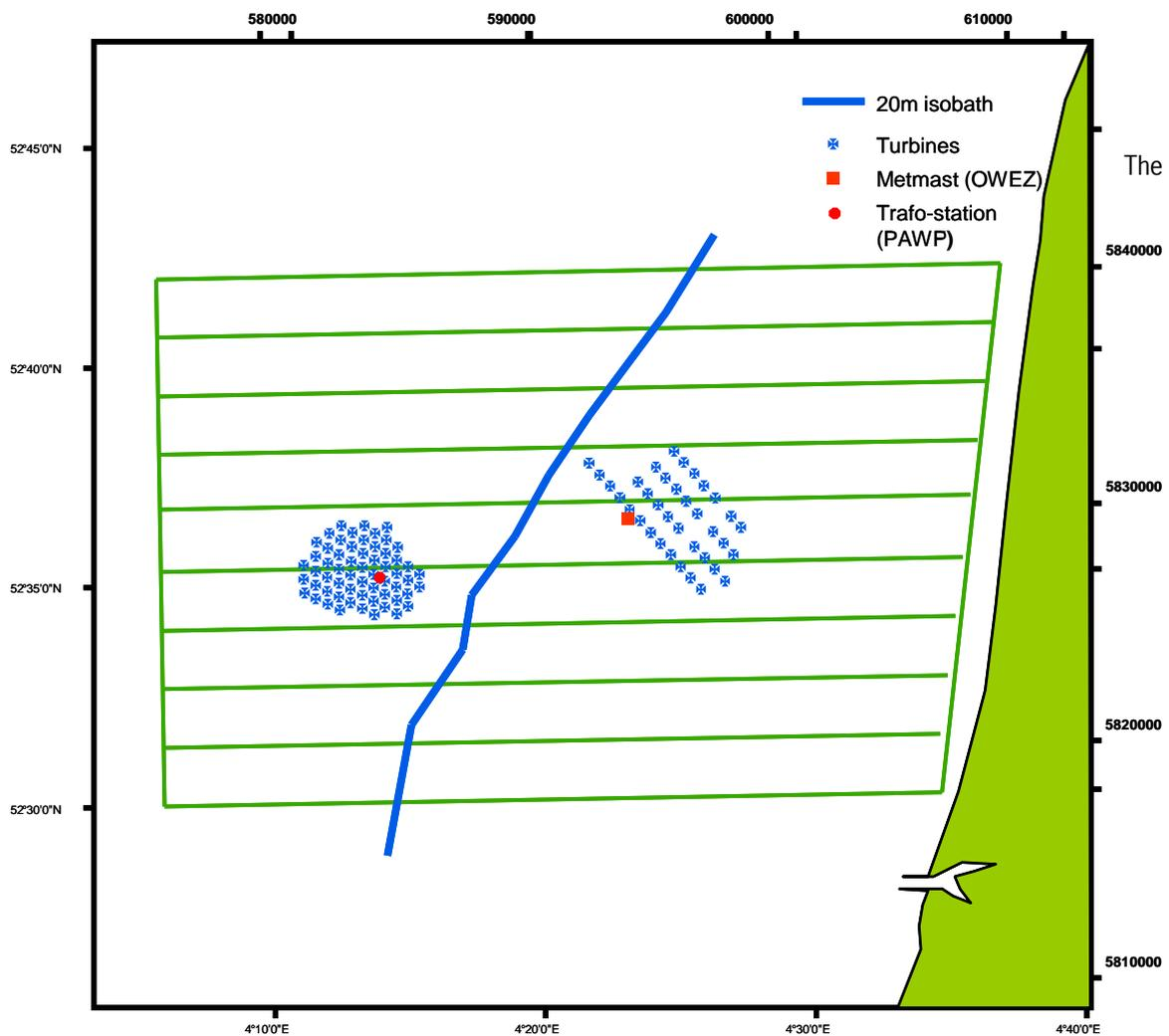
**Figure 8.** Location of OWEZ with 36 turbines and of PAWP with 60 turbines, to the northwest of the port of IJmuiden. The two wind farms are situated on either side of the -20 m isobath (blue thick line). In addition to the turbines, OWEZ has a 116 m high met-(meteo)mast situated on the seaward side of the wind farm, and PAWP has a transformer platform within the wind farm (both indicated by red symbols). The green lines running E-W are the principal survey lines (see methods section).
