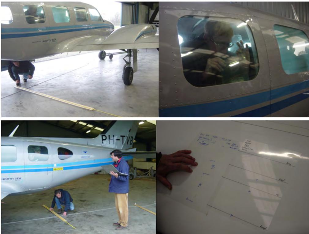
Calibration of observer and side specific strips for the two-engine survey aeroplane PH-TVB during an annual ground truthing session. In the upper right picture an observer is determining his strip by drawing his inner, middle and outer line of his strip. Based on goniometric calculations the strip can be determined and compared with the goniometric calculations of the strip measured on the floor of the hangar.
