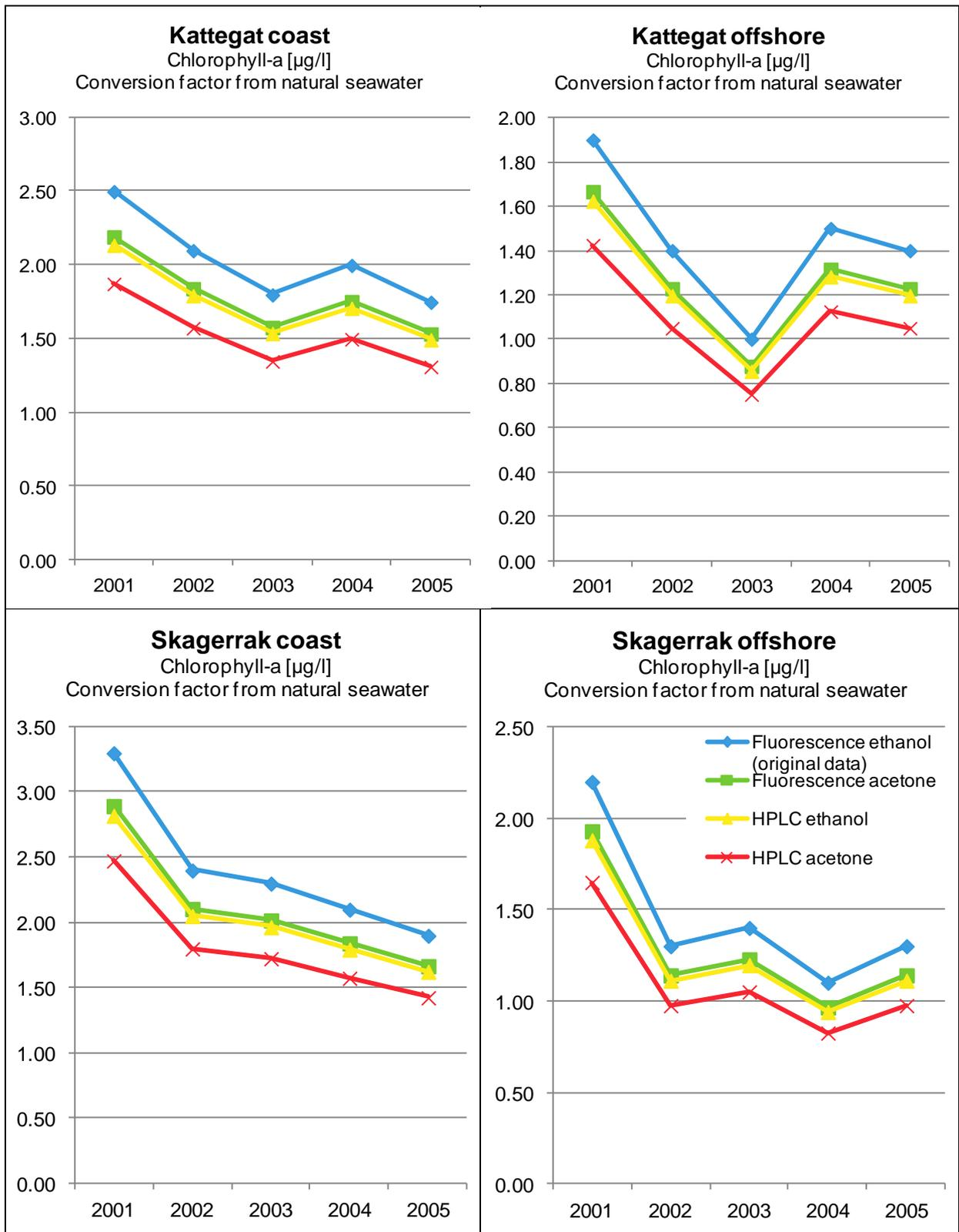
Fig 7. Seasonal means (2001-2005) of chlorophyll-a used in the Swedish national report for the OSPAR Assessment 2007. Swedish chlorophyll data are analyzed with fluorimetry and ethanol as extraction (original data). Data are then “converted” to fluorimetry/acetone, HPLC/ethanol and HPLC/acetone using Quasimeme test data from natural sea water.
