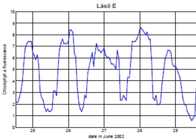
Fig. 1 Variability of *in vivo* chlorophyll fluorescence measured at approximately 2 m depth using the SMHI oceanographic buoy Läsö E. in the Kattegat in 2002. Night time to day time ratio is about 2-3.
