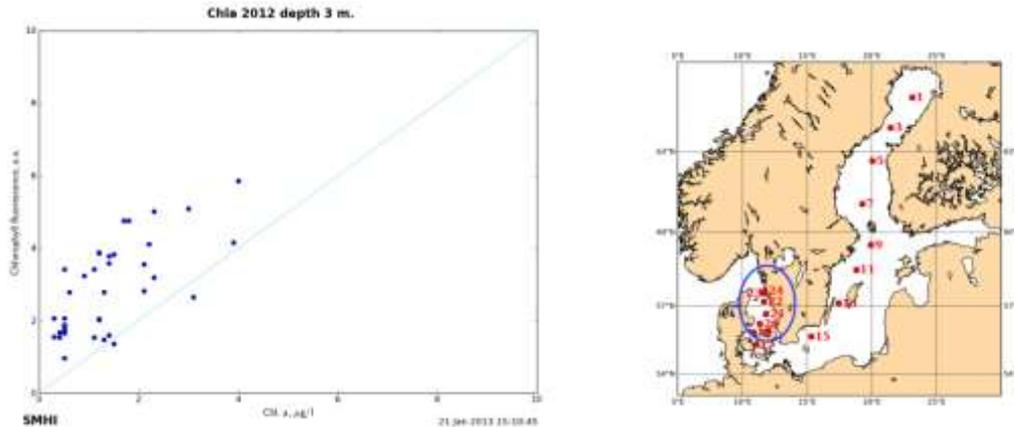
Fig. 3. The correlation between *in vivo* chlorophyll fluorescence and extracted chlorophyll from water samples, measured at approximately 3m depth on a FerryBox system in the Kattegat and Skagerrak area in 2012.
