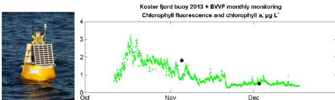
Fig. 2 *In vivo* chlorophyll fluorescence in the Kosterfjord in 2013 measured at approximately 1 m depth. Black dots represent water samples for chlorophyll a analysed in the laboratory as part of the regional monitoring program (BVVF).
