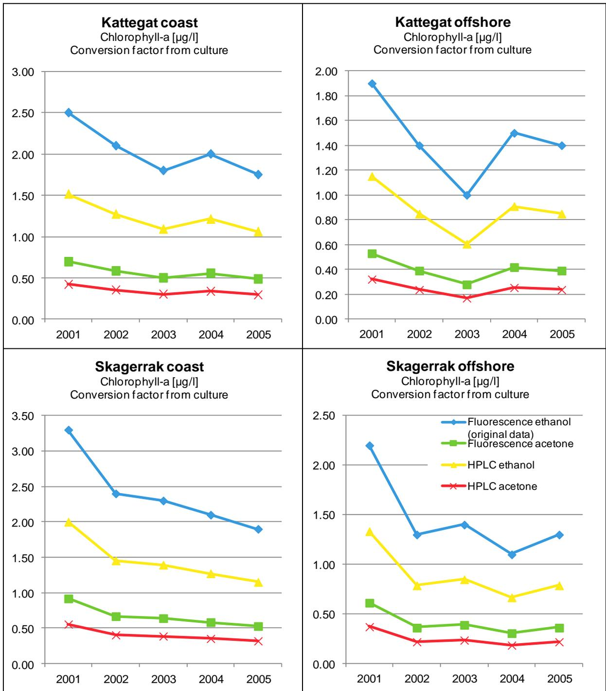
Fig 8. Seasonal means (2001-2005) of chlorophyll-a used in the Swedish national report for the OSPAR Assessment 2007. Swedish chlorophyll data are analyzed with fluorimetry and ethanol as extraction (original data). Data are then “converted” to fluorimetry/acetone, HPLC/ethanol and HPLC/acetone using Quasimeme test data from culture.
