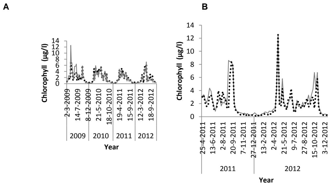
Fig 6. Comparison of weekly uncorrected chlorophyll concentrations determined by fluorometric methods (grey line) and chlorophyll 'c2' determined using HPLC (dashed line) at the (A) Stonehaven and (B) Loch Ewe monitoring sites.
